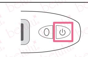
How to turn off the product is to push the power button over 3 seconds.
