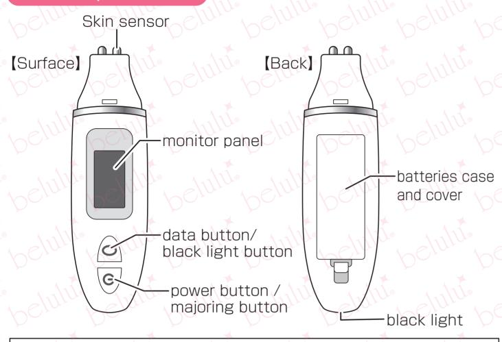
Size: H122×W34D25mm Weight:37g(without battery) Using battery: AAA battery×2 Recommend temperature/humidity:  $5^{\circ}$ C~40°C/under 70%
